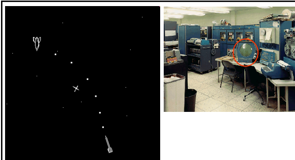
SPACEWAR: the original video game first realized on the MIT PDP-1 in 1962 PDP-1 – 100KHz, 4K RAM, $100,000
